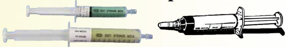
**Diamond Compound** is available in 5-gram and 10-gram syringes that make application easy. Graduated marks along the side of the syringe indicates amount. Apply the compound in tiny dots and spread evenly across the pad, add a few drops of diamond extender fluid and spread with a fingertip. Rotate the part being ground and check frequently for overheating. Add a drop of extender fluid to cool off the work piece. Recharge the plate only when necessary as the diamond lasts a long time.
