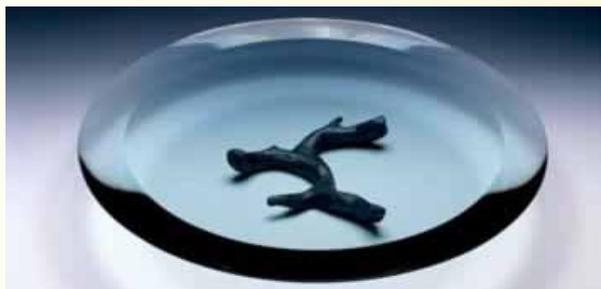
*NOTE: The Covington Plate Dresser is an excellent tool to keep your Rociprolap® plate running true. The sintering on the diamond dresser provides fast removal of uneven spots on the plate. This dresser also works well on other plate machines.*
