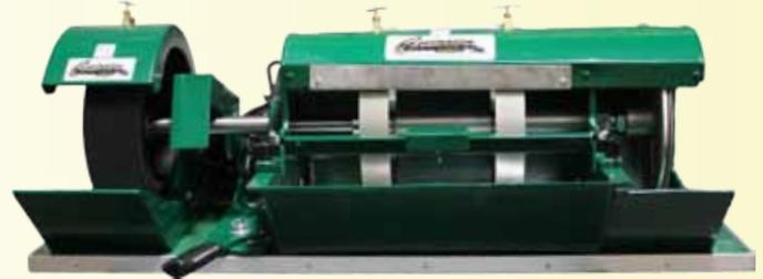
The #754 8" Diamond Grinder/Polisher comes with two 8" x 1-1/2" metal bond diamond grinding wheels (100g & 220g), two 3" x 25-7/32" diamond cloth belts (400g & 1200g), one 8" x 1"-14RH aluminum head with leather disc attached, a 5-gram syringe of 50,000 mesh diamond compound, a 2-ounce bottle of extender fluid, sample kit (polish powder, brush, dop sticks, and wax), a book about using diamond abrasives, instructions, and product guarantee.
