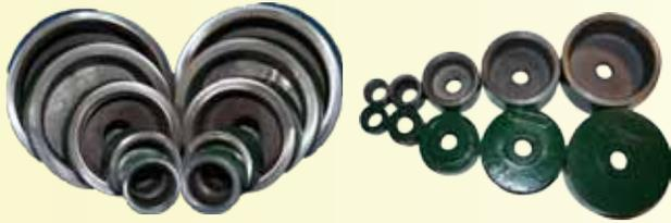
Covington's Cast Iron Cutter Cups are designed to provide maximum grinding surface contact while allowing for imperfections in the preformed spheres. The soft cast iron material allows the grit to embed itself in the cutter cup, promoting a faster grind. These high quality cups are preferred and used by many lapidary and glass artists.
