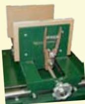
This book-end type vise holds work pieces of any shape tightly, but quick-release feature allows an easy, no-bind return. The steel jaw tongue contacts the full length of the vise, holding the jaw square so it can't bind. The end grips have a hardwood facing. A cross shaft is included with each vise.
