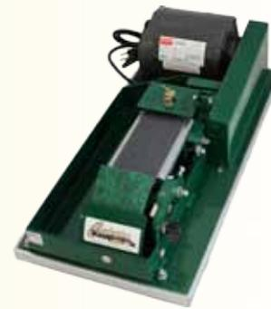
The #460 Horizontal Wet Belt Sander is designed for grinding flat surfaces such as tiles. This sander uses 3" x 25-7/32" sanding belts and comes complete with a 1/3hp motor mounted on a rustproof aluminum-topped Lam-I-Cushion base, a water valve and spray nozzle for water supply hookup, 3" x 6" backing plate, instructions, and product guarantee. This machine ships with the motor attached, ready to plug in and operate.
