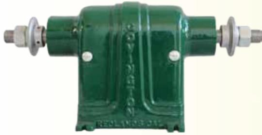
The **Two-Station Closed Arbor** is a low cost “build-your-own” style grinder/polisher. This versatile unit is designed to accept 6”, 8”, and 10” wheels. The arbor ships with two (2) nuts, 3” drive pulley, v-belt, and two (2) sets of 3” diameter flanges. The split housing, with a closed center, connects using two bolts. Two bearings are set on the shaft with two set screws. This arbor can be disassembled and reassembled in minutes.
