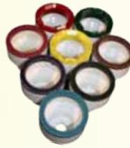
The 4" Diamond Cutter Cups grind faster than conventional silicon carbide cutter cups. The Sintered Diamond Cutter Cups, manufactured in house, are aggressive without being harsh and accommodate spheres from 3-3/4" to 6-1/2". The Resin Bonded Diamond Cutter Cups provide better control and grind quickly. These are designed for finishing spheres. All cutter cups come with 3/4" National Pipe Thread.
