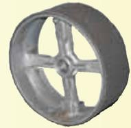
Covington's Lever-Lock Drums are made of sturdy cast aluminum and balanced to reduce vibration. The 3" rim is covered with sponge rubber. The lock area is threaded for setscrew-operated clamp, just loosen to remove the old cloth and retighten to secure the new. This drum comes with a 220g wet/dry sanding cloth installed. \*Specify bore size when ordering, 1/2", 5/8", 3/4", or 1".
