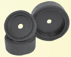
Covington's Expandable Drums feature angled slots through the heavy rubber rim which allow the drum to expand when rotated, thereby locking the belt in place. Belts can be quickly changed by stopping the machine, slipping off the old one and sliding on the new one. In use, the resilient drum surface flexes to the gemstones contour to quickly remove grinding flats. Run at a maximum speed of 1725rpm.
