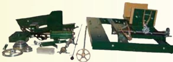
The Carriage Slab Saw Kit is a "build-your-own" style unit that requires the user to construct a tank. This kit comes complete with a saw frame, carriage and vise assembly, arbor, blade guard, rock catcher, and power feed assembly. The carriage assembly ships mounted on the guide ways within the saw frame.
