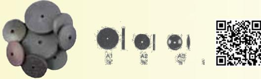
Cratex Wheels are individual rubber bonded abrasives for polishing, removing rust, etc. These wheels are available in 3 grits: coarse (green), medium (brown), fine (reddish-brown), and fit M-1 or M-6 mandrels. Maximum speed rating of 25,000rpm.
