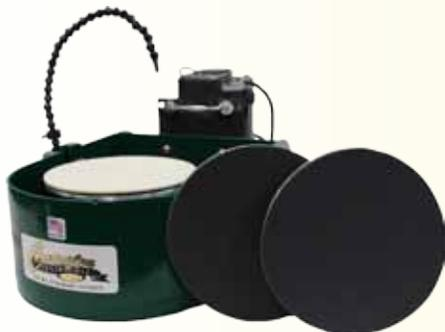
The #5070 **8" Standard Maxi Lap** comes with three (3) 8" x 1/2"-20RH thread quick-change aluminum heads and Covington's fast cutting silicon carbide abrasive system. The standard kit includes: two (2) 8" x no arbor hole silicon carbide sanding discs (100g & 400g), and one (1) 8" x no arbor hole 1/8" thick felt polishing disc. All discs are affixed to a hard rubber face with "Stick-N-Peel" adhesive.
