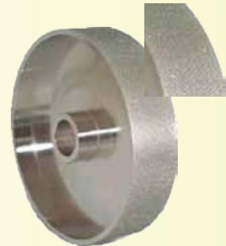
Covington's 6" and 8" **Textured Grinding Wheels** are excellent tools for pre-forming rough stone and glass material. The texturing allows for better sediment wash-out. These balanced, solid steel wheels, are nickel electroplated to provide superior bonding of diamonds and a long life.
