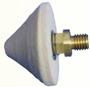
Felt Cones are an excellent choice for working bottles and inside curves. These cones are approximately 3" at base and 3" in height. The felt cones come with a 5/8"-11 male brass thread to fit a 5/8"-11 female thread. Use in combination with cerium oxide to achieve a high, optically-clear polish.
